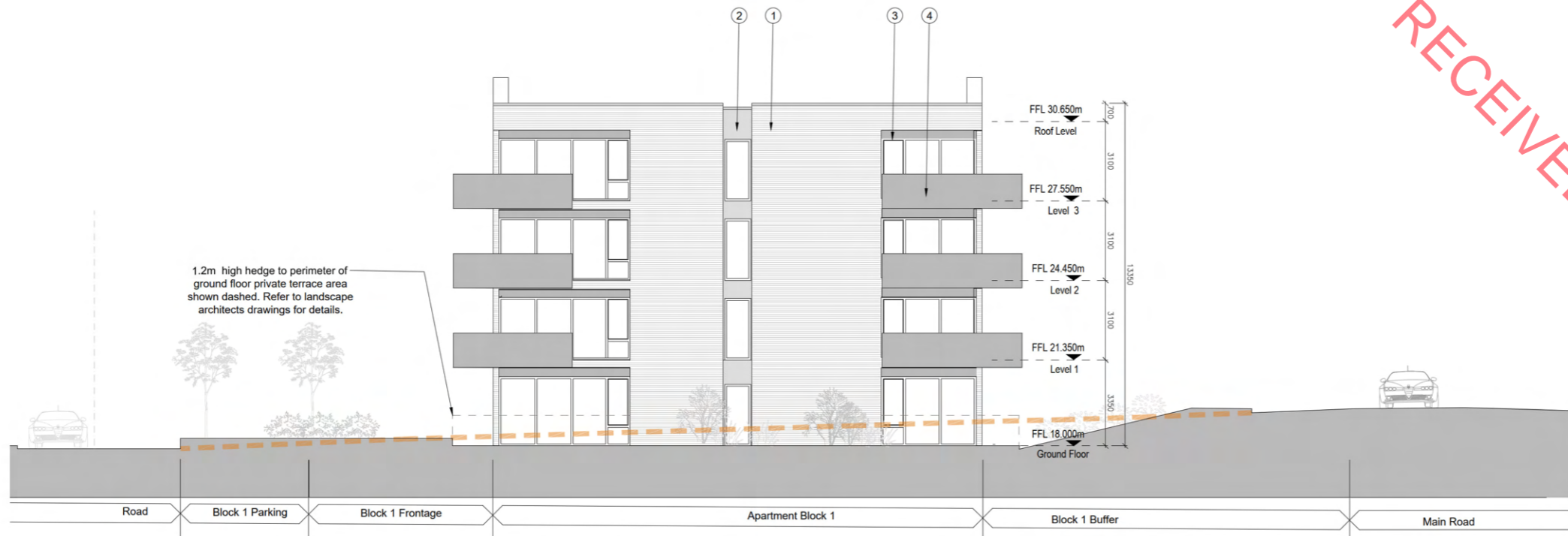
02 Elevation facing South APARTMENT BLOCK 1 SCALE: 1:100
